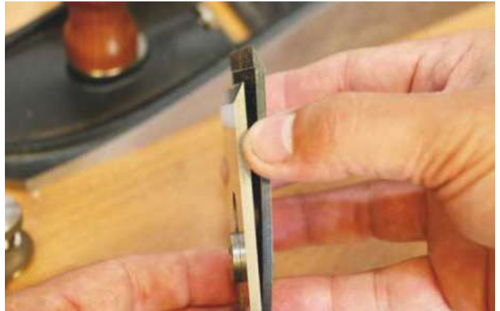
▲ Alternatively you can slacken both screws to let the irons slide apart
